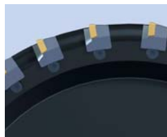
Differential pitch reduces vibration.
